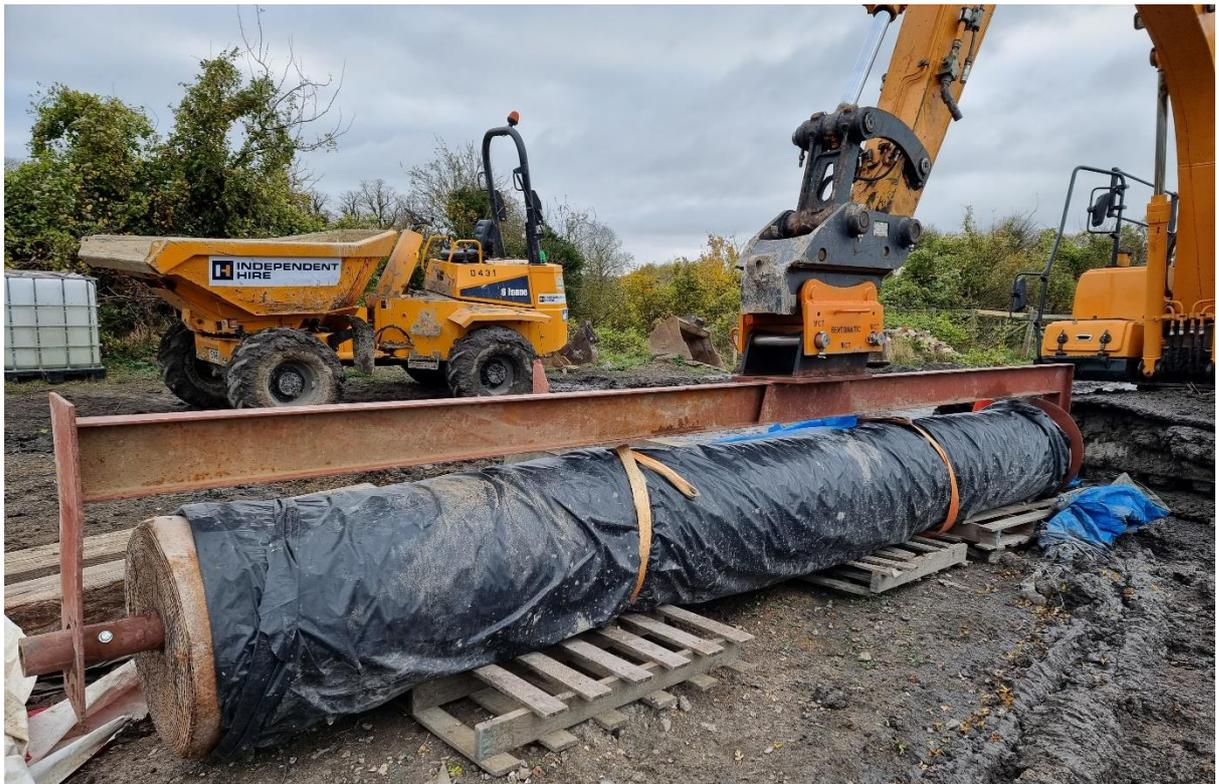
Bentomat dispenser. Note quick-hitch adapter plate and securing bolt under top bracket (on left).
