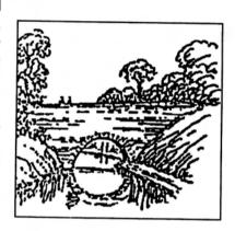
The steep, shrub clad, bank leading to the road above is the site of Little Tring Bridge. This was infilled in the early 1970's as part of a national exercise to make road bridges strong enough to take the heavier weight lorries that were going to be allowed on Britain's roads in the name of progress.
