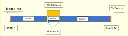
A control weir has been built into the earth dam at Bridge 4a to allow control of the water flowing into the section of canal. On 15<sup>th</sup> June water was let back into the section of canal starting at Bridge 4a, with the sluice gate at Whitehouses placed in the open position. The intention was to rewater section 1 and to ensure that the block wall was watertight.
